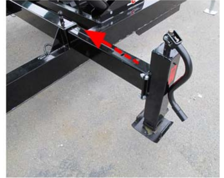
Slide the outrigger towards the trailer until the pop-pin locks back into place.
