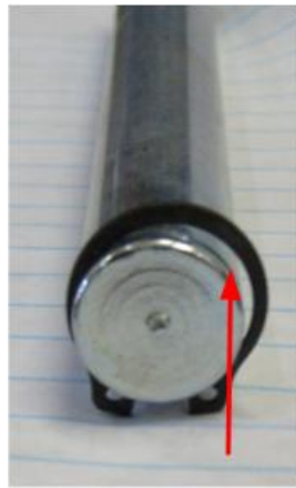
WRONG Gap between snap ring and pin
