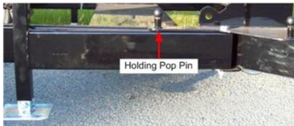
Space Saver 1 Style Rear Swing Arm Jack Forward in Travel Position
