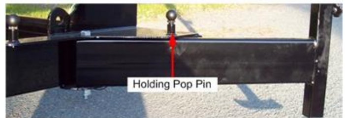
Space Saver 1 Style Rear Swing Arm Jack Rearward in Raising/Lowering Position
