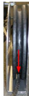
2. Lay pulley on top of cable with cable in groove of pulley
