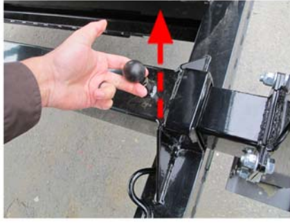
Pull up the pop-pin to allow the outrigger to slide back towards the trailer.
