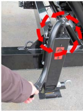
Turn jack handle counter-clockwise until you no longer can raise the jack.
