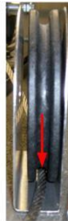
2. Lay pulley on top of cable with cable in groove of pulley
