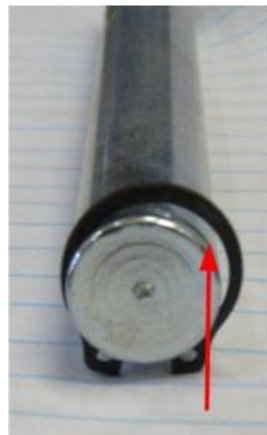
WRONG Gap between snap ring and pin
