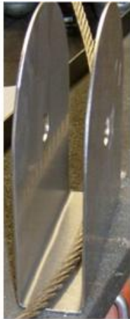
1. Lay cable through davit shield
