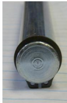
CORRECT No gap between snap ring and pin
