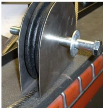
3. Bolt with washer through hole in shield and pulley
