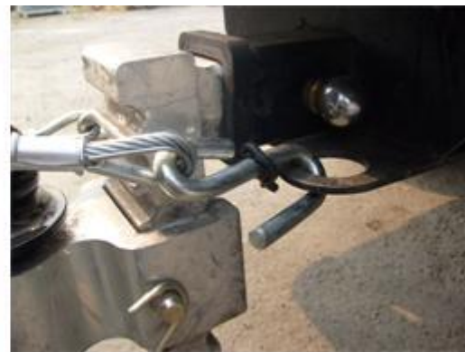
Right Side Safety Cable
