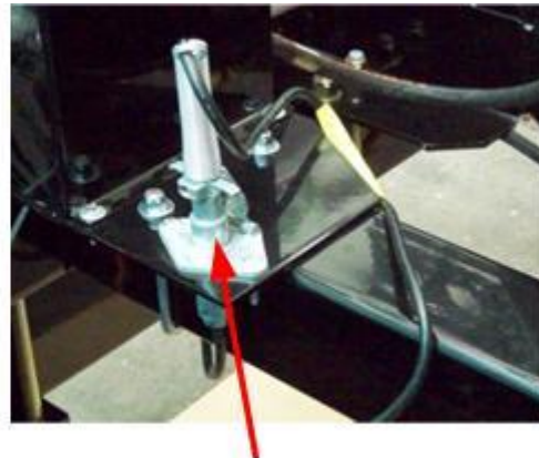
Lift Controller Plug Inserted into Socket
