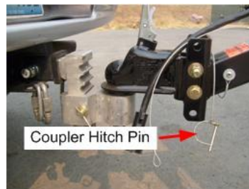
Coupler Hitch Pin attached to towing tongue with lanyard.
