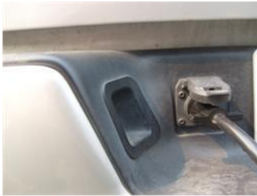
Electrical Towing Plug properly inserted into tow vehicle socket with socket cover safety catch down over trailer plug
