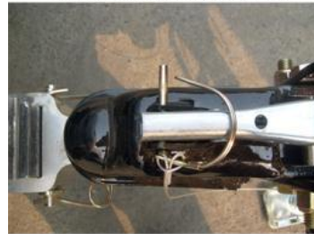
Slide the Coupler Hitch Pin Clip over the end of the pin to lock in place.
