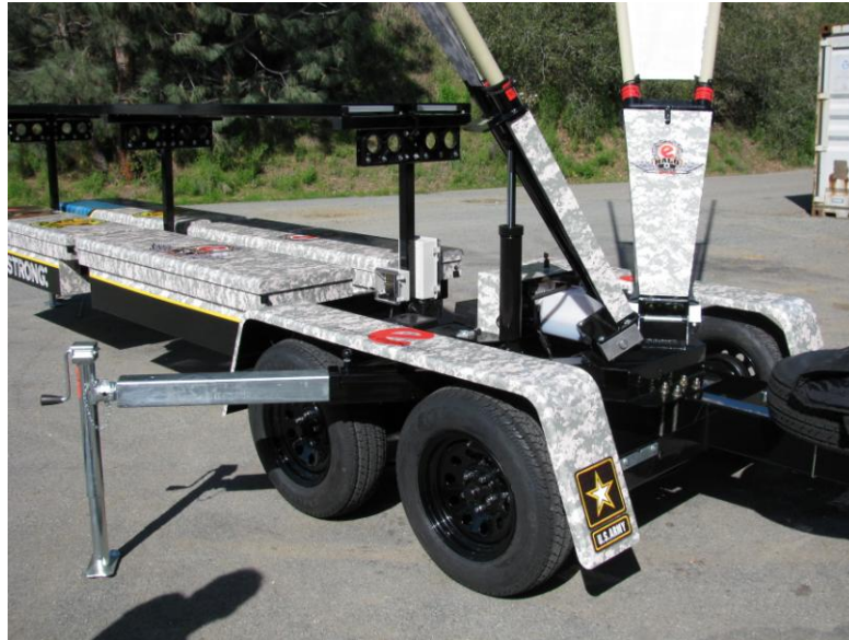
Proper positioning of Stabilizer Arm and Jacks for operation.
