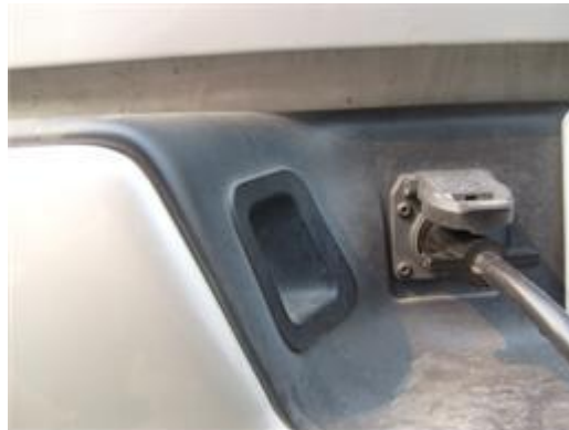
Electrical Towing Plug properly inserted into tow vehicle socket with socket cover safety catch down over trailer plug
