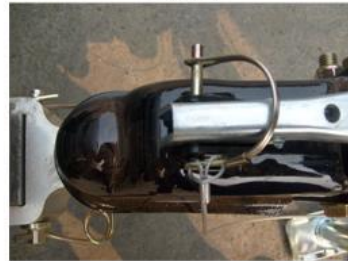
Proper installation of Coupler Hitch Pin and Hitch Pin Clip set for towing.
