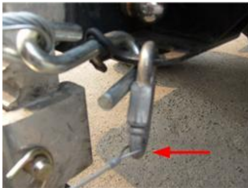
Emergency Brake Break-A-Way Lanyard Attachment
