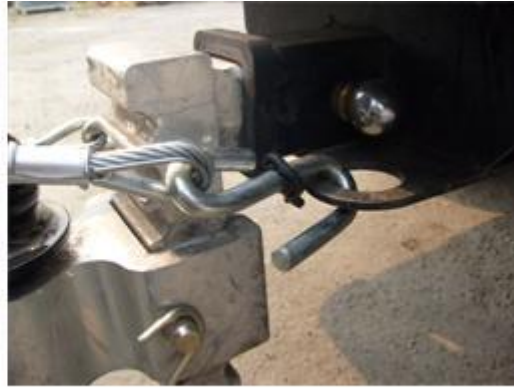
Right Side Safety Cable
